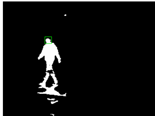
Figure 6: The bounding box of the head region. I draw it a little larger than it should be to make it noticeable.
